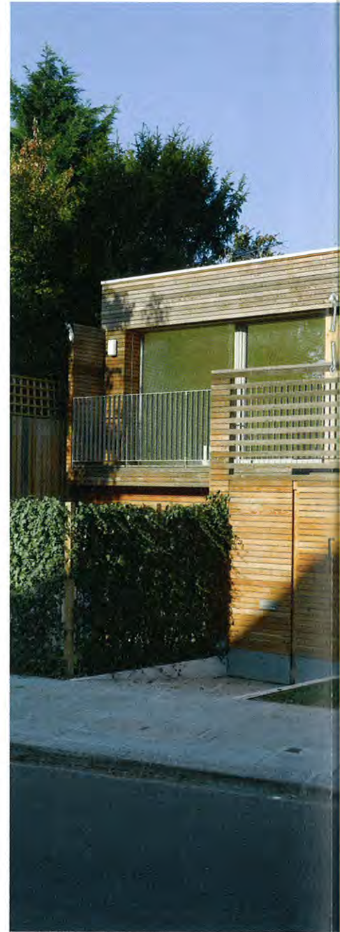
3 Open courtyard in north-west corner The north west courtyard results in a high percentage of glazing not south-orientated. Again, the TFA is too high. Result = 16.7 kWh/(m 2 a)
