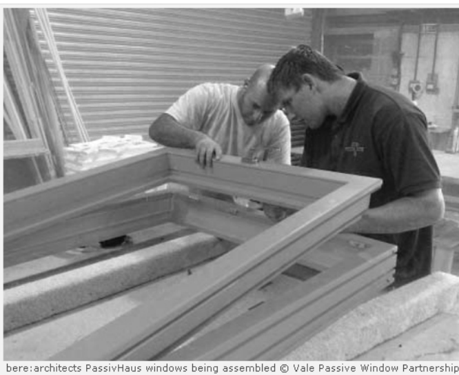
bere:architects PassivHaus windows being assembled © Vale Passive Window Partnership
