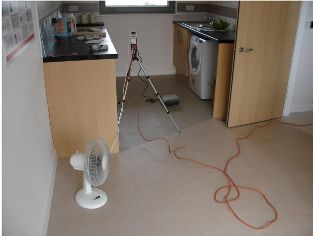
Temperature monitoring equipment set up in Larch House during the co-heating test
